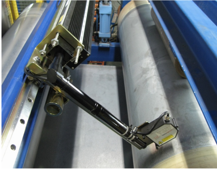
Early prototype of Wolf DFM1 Dry Film Thickness Monitor showing CO2 laser at the top and the laser sensor in the foreground.
